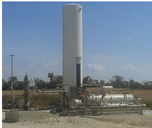
Figure 8. The CO 2 system and 22 ton tank (September, 2015).
