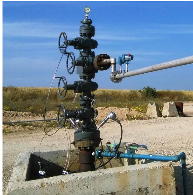
Figure 16. Wellhead of the injection well H18A.
