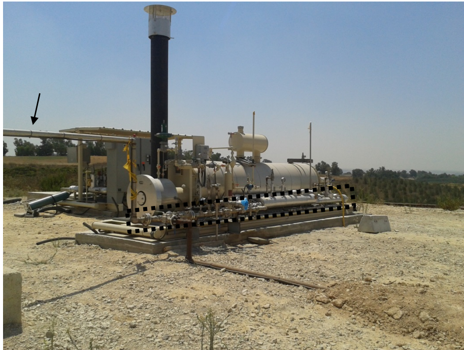
Figure 7. The CO 2 heater and manifold sections. The manifold is a junction for batch tracers and water tube with CO 2 fluid (black frame). The manifold is connected to the wellhead (black arrow). Tracer injection
